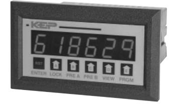
Input Impedance: Current:  $100\Omega$ ; Voltage:  $115K\Omega$ Overvoltage Protection: 50 V Overcurrent Protection: 50 mA Resolution: 14.5 Bits
